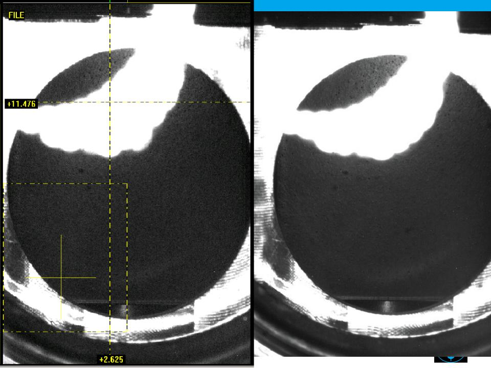
Charge 500 pC at 27.87 MeV/c | Imain= 394 A (focus + 2A) | BSA of 1.2 mm, (3/21\3 ps)
