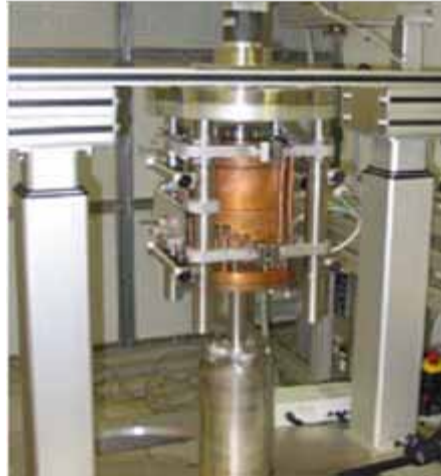
Vertical cleaning setup with 110° rotating nozzle.
