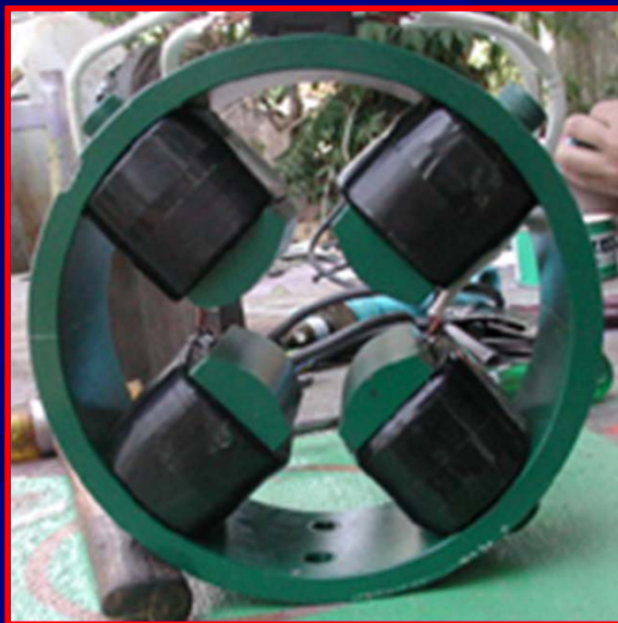
completed quadrupole magnet
