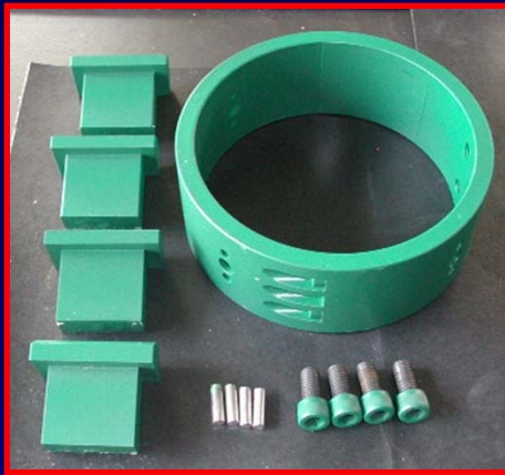
quadrupole magnet poles & coils & frame
