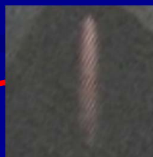
Image of electron beam at view screen downstream of dipole magnet
