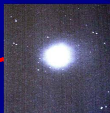
Image of electron beam at the end of beamline
