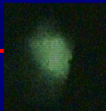
Image of electron beam at transition radiation station
